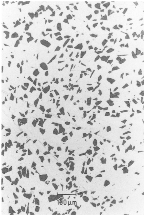
Figure 8 Region of well-distributed particles in a 30 \mu\text{m} SiC particle-commercial-purity magnesium composite produced by pressure infiltration and dispersion into more metal. The volume fraction of SiC is 16%.
