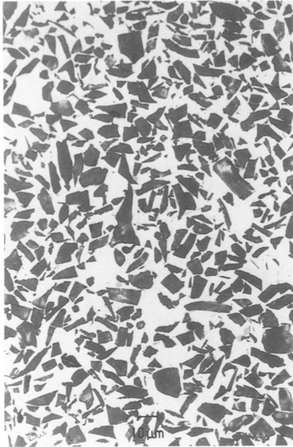
Figure 6 Typical microstructure of a 10 \mu\text{m} SiC particle-commercial-purity magnesium composite produced by pressure infiltration. The volume fraction of SiC is 48%.
